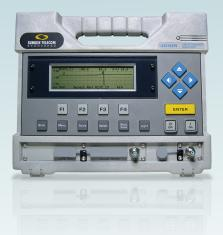
This portable battery-operated instrument includes forward sweep, return sweep, and signal-level meter (SLM) capabilities. With option 052 (forward sweep transmitter) installed it can also function as a headend unit for troubleshooting intermittent problems in specific network segments. It incorporates Digisweep technology, the fastest high-resolution sweep, allowing placement of sweep points close to digital signals without interference.
