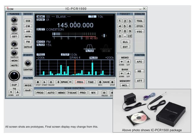
Icom proudly announces the debut of the IC-PCR1500. This computer-controlled receiver is the successor of the IC-PCR1000 and designed for scanner enthusiasts or professional users who monitor various channels. It covers from 0.01 to 3299.999MHz in all modes (0.495-1300MHz only in SSB and CW modes) and versatile functions such as multi-channel monitor, bandscope and IF shift function support efficient and effective reception.
