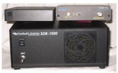
Figure 2 - FlexRadio SDR 1000 Transceiver with RFSpace SDR-14 and ICOM PCR1000 receivers sitting on top.
