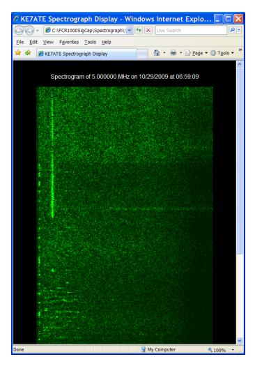
Copying the recorded files to another folder will allow you to save the files for future review and analysis. The screenshot shown above shows an example of capturing the sub-audible time code of WWV. The waterfall display is calibrated with a tick mark every 250 Hz allowing quick estimation of peak frequency. You can also use the Data Explorer feature to show the approximate peak frequency in the spectrum display.
