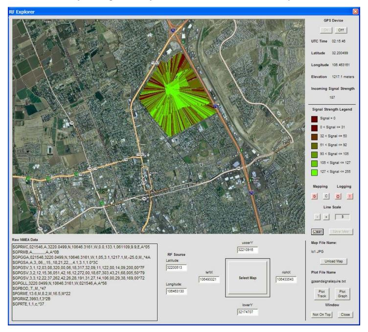
Map an RF Source such as a transmitter site and collect signal data in relation to incoming GPS data.
