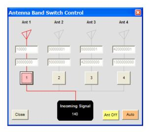
Antenna Band Switch. Frequency ranges may be set according to your antenna receive ranges.
