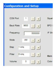
Also, you may set display colors and have specific windows open when the receiver is turned on, you may even have the Explorer tools open. Other settings include options to set the optional hardware to connect to specific COM ports as needed. You may even select the type of s-meter you want to use on startup.
