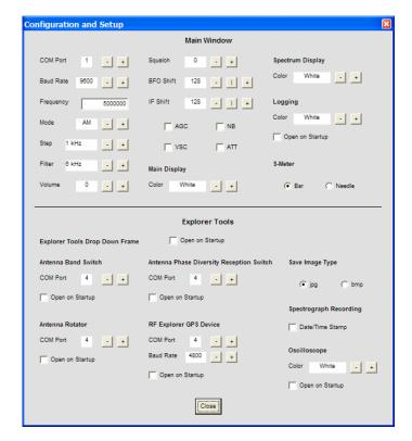
Configure your software to startup with a preferred frequency, mode, step, or filter setting. Adjust the startup volume, squelch, IF and BFO Shift controls to whatever startup setting you need when you turn on the IC-PCR1000 communications receiver. The COM port setting may be set to the serial port your receiver is connected and the baud rate is set to whatever baud rate the receiver has been set to use.
