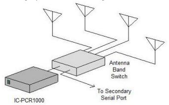
Expand your antenna input to automatically select an antenna suited to your received frequency range. Connect up to four antennas of your choosing via the antenna connectors on the
