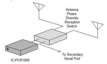
All antenna options require a secondary serial port installed on your computer and the appropriate antennas to utilize the optional hardware. The Antenna Band Switch, Antenna Phase Diversity Reception Switch and Antenna Rotator are available pre-assembled and pre-tested. Contact me for pricing and information if you are interested in expanding the antenna connector on your IC-PCR1000 communications receiver.
