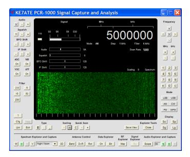
Record the waterfall display and view it using your system's default web browser. This unique feature is terrific for storing spectrographic information about a signal and may be date/time stamped as needed. The length of recording is only limited to the free space you have on your hard drive.
