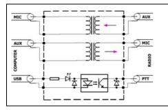
Input and output audio signals from the radio to the computer and vise versa are supplied through 1:1 bidirectional audio transformers for proper isolation of the circuit.
