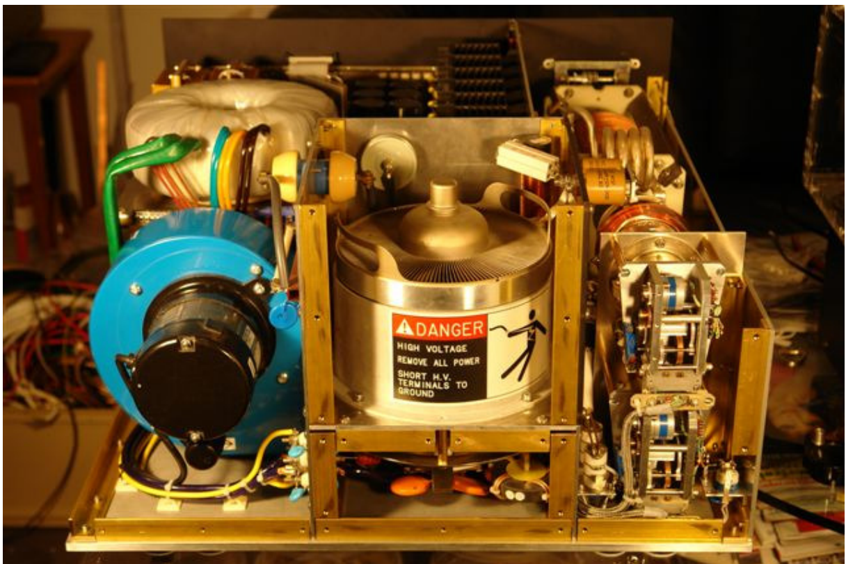
Fig. 10: Power amplifier without back board, the motors for the two vacuum capacitors on the right
