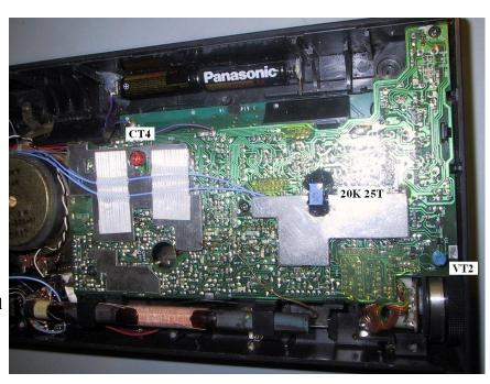
frequency (the beat note is louder and easier to hear in one or the other of USB or LSB depending on whether you are tuned higher or lower). If necessary, adjust the pot so that the beat notes are about the same frequency when you are tuned 0.1 to 0.3 kHz higher and lower. Some may find it easier to adjust zero beat with a station playing music.
