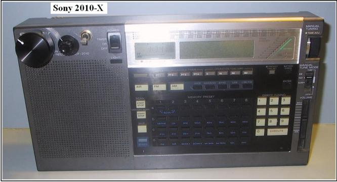
The photo above shows a front panel view of the finished tuned whip mod. The knobs are somewhat cramped, but then there is not much space for a DPDT toggle switch, a rotary switch, and potentiometer. The NKK MRX204A rotary switch knob came with the switch. The switch shaft was longer than necessary and was cut shorter with the cutting wheel of a Dremmel tool. The knob is a modified (small hole drilled and indicator line and hole painted white) black anodized Eagle (EPD) knob, Mouser # 450-6008.
